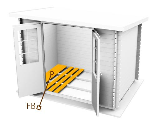
SAW THE BASEBOARDS AND ATTACH WITH NAILS AT EVERY 0,5 METERS.
